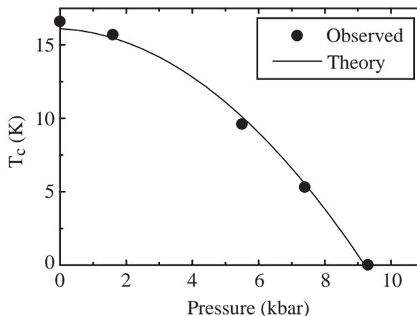
Fig. 1. Pressure dependence of Curie temperature in TDAE-C<sub>60</sub>. Closed circles represent observed value. Solid line indicates the simulation result based on the orbital ordering model.
