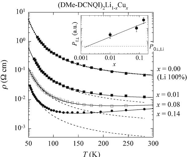
Fig. 3. The temperature dependence of the electrical resistivity reproduced by the hole soliton model in several Cu concentrations. Closed squares are taken from the reported resistivity in Ref. 1. The solid curves show the hole soliton model,  $\rho = \rho_{\parallel} + \rho_{\perp}$ . Dashed curves represent  $\rho_{\perp} = \{\sigma_{0\perp} \exp(-260/T)\}^{-1}$ . Inset shows  $P_{0\perp}$ .
