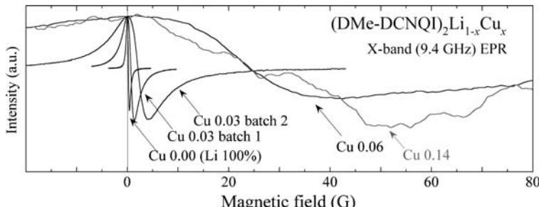
Fig. 1. Derivative EPR spectra taken at X-band in single crystals of  $(\text{DMe-DCNQI})_2\text{Li}_{1-x}\text{Cu}_x$  ( $x \leq 0.14$ ). The abscissa is measured from the positive peak of the spectrum.
