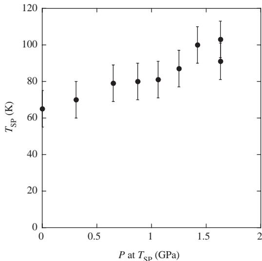
Fig. 1. The pressure dependence of  $T_{SP}$  for the Li salt.
