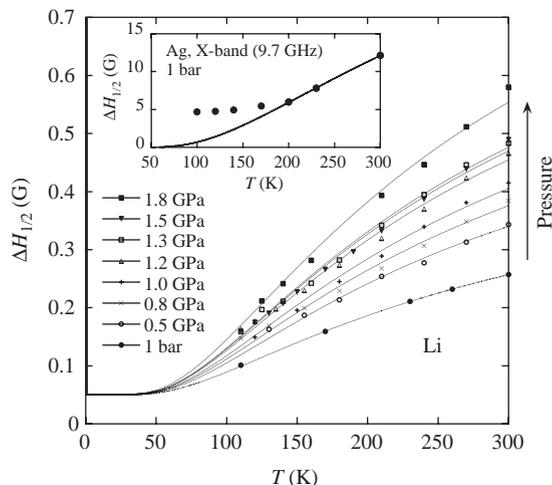
Fig. 2. Temperature dependence of ESR linewidth taken at 50 MHz in the powder Li salt above  $T_{SP}$  with implicit parameter of hydrostatic pressure up to 1.8 GPa. The inset shows the linewidth for Ag salt at X-band and ambient pressure. Solid lines represent an empirical formula,  $0.05 + A(P)\exp(-250/T)$  for the Li salt and  $B(P)\exp(-400/T)$  for the Ag salt, where  $A(0) = 0.5$  G and  $B(0) = 50$  G.
